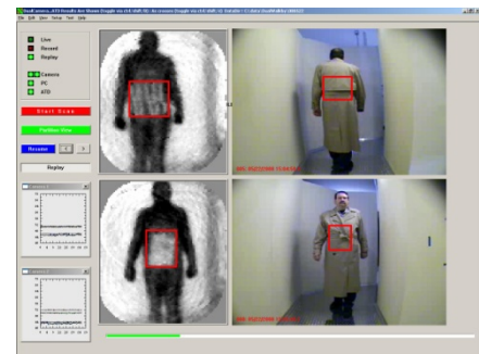
Figure 3. Active Millimeter Wave Detection Portal Images
